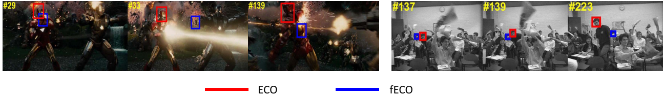
Fig. 13. Failure cases of the proposed method. The videos are Ironman and Freeman4 from OTB-2015 [10]. Our compressed model struggles when an occlusion or a drastic appearance change occurs.
