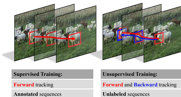
Figure 1. The comparison between supervised and unsupervised learning. Visual tracking methods via supervised learning require ground-truth labels for every frame of the training videos. By utilizing the forward tracking and backward verification, we train the unsupervised tracker without heavyweight annotations.
